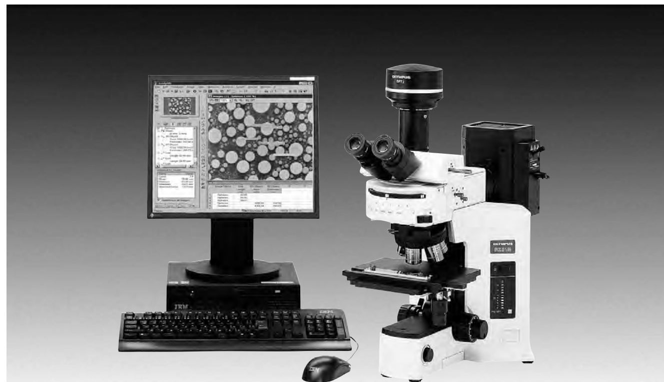
Sample combination with an industrial microscope and a digital camera
